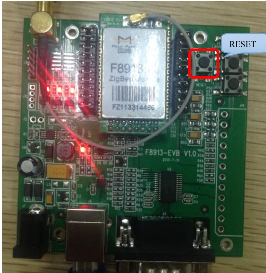
figure 2-9 The “reset”button on the development board
