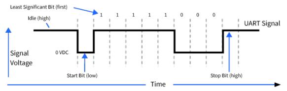
You can configure the UART baud rate, parity, and stop bits settings on the device with the **BD**, **NB**, and **SB** commands respectively. For more information, see UART interface commands.
