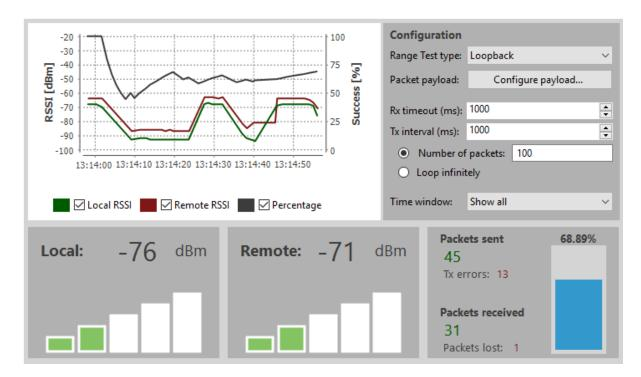
8. Move Radio 1 around to see the resulting signal strength at different distances. You can also test different data rates by reconfiguring the **BR** (data rate) parameter on both radios. When the test is complete, click **Stop Range Test**. XCTU displays another loopback jumper warning screen reminding you to put the loopback jumper back in its original position.
