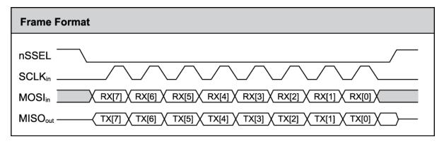
SPI mode is chip to chip communication. We do not supply a SPI communication interface on the XBee development evaluation boards included in the development kit.
