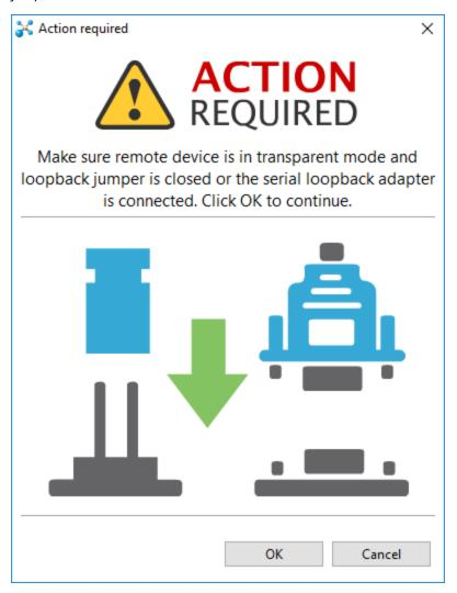
Plug in the XBee3 802.15.4 RF Module has pictures that show the jumper in the UART position—move the jumper to the left on the surface-mount device or down on the throughhole device puts it in loopback mode
